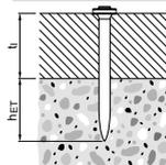
$L_s = h_{ET} + t_1 \text{ [мм]}$
