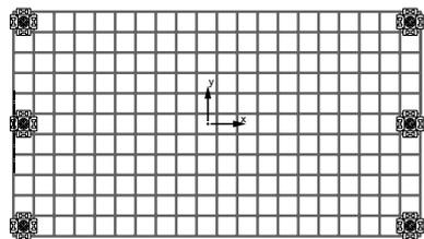
$$V_{GR,y,Rd} = 2 \cdot n \cdot V_{Rd,a} \\ = 2 \cdot 3 \cdot 4.5 = 27.0 \text{ кН}$$
